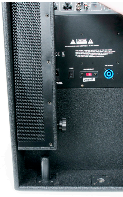
When the screw is loose enough, remove the array speaker from the base.
