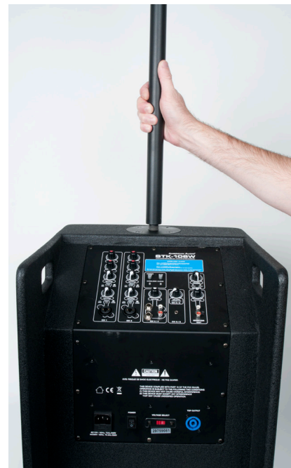
Screw the array speaker pole into the top of the subwoofer.
