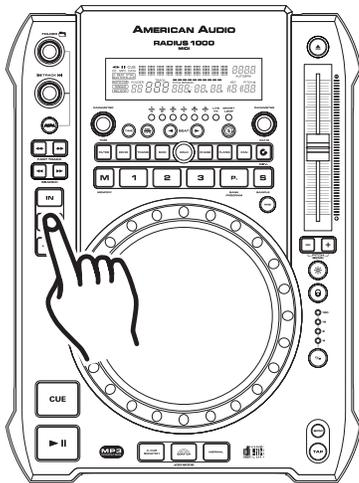
3) Press the *OUT BUTTON (15)* to set the ending point for your SEAMLESS LOOP (Figure 20). The *IN BUTTON (15)* and *OUT BUTTON (15)* LEDs will immediately begin to flash rapidly, indicating the SEAMLESS LOOP mode has been activated.
