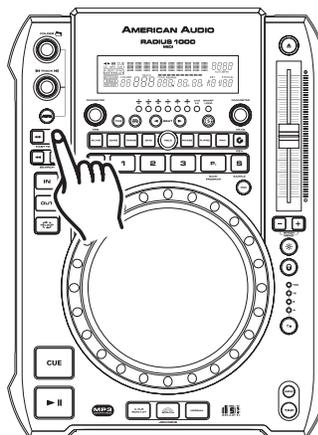
**Figure 8:** Tapping the forward track button or turning the track knob clockwise will skip forward to the next track.
