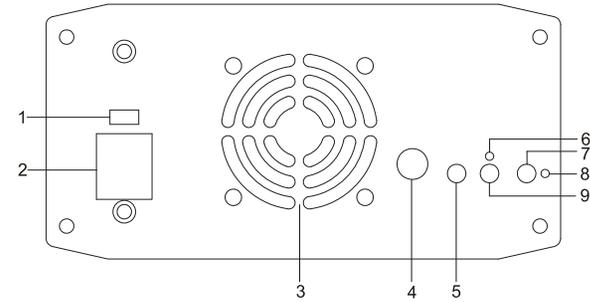
1. Power Switch - This switch powers the fixture on/off.
