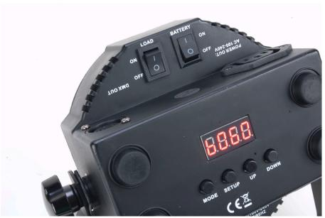
To charge the battery, connect the unit to AC power, and put the Battery switch into the "ON" position. The display will begin to flash and show the battery life percentage.
