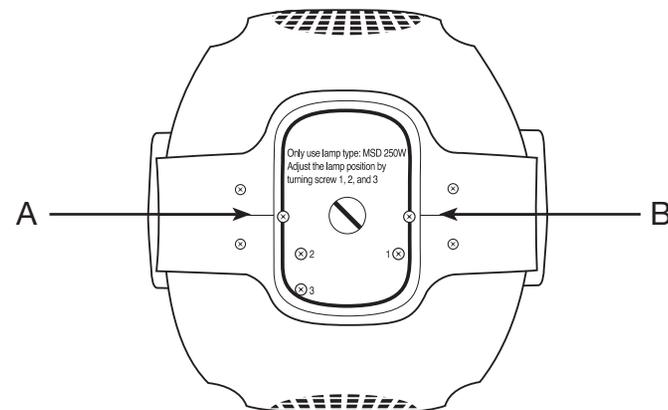
**Accu Spot 250 II™ Fuse & Lamp Alignment**
