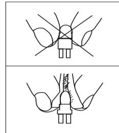
This fixture is fitted with a discharge lamp which is highly susceptible to damage if improperly handled. Never touch the lamp with your bare fingers as the oil from your hands will shorten lamp life. Also, never move the fixture until the lamps have had ample time to cool. Remember, lamps are not covered under warranty conditions.
