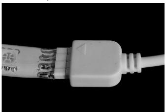
When making the connection to the Accent Strip, follow the arrows located on the connector. With the Accent Strip facing up, make sure the the arrow located on the connector is at the top and facing the Accent Strip. Please see above pictures. Continue connecting Accent Strips in the same way. If you connect in strips any other way, they will not sync up.
