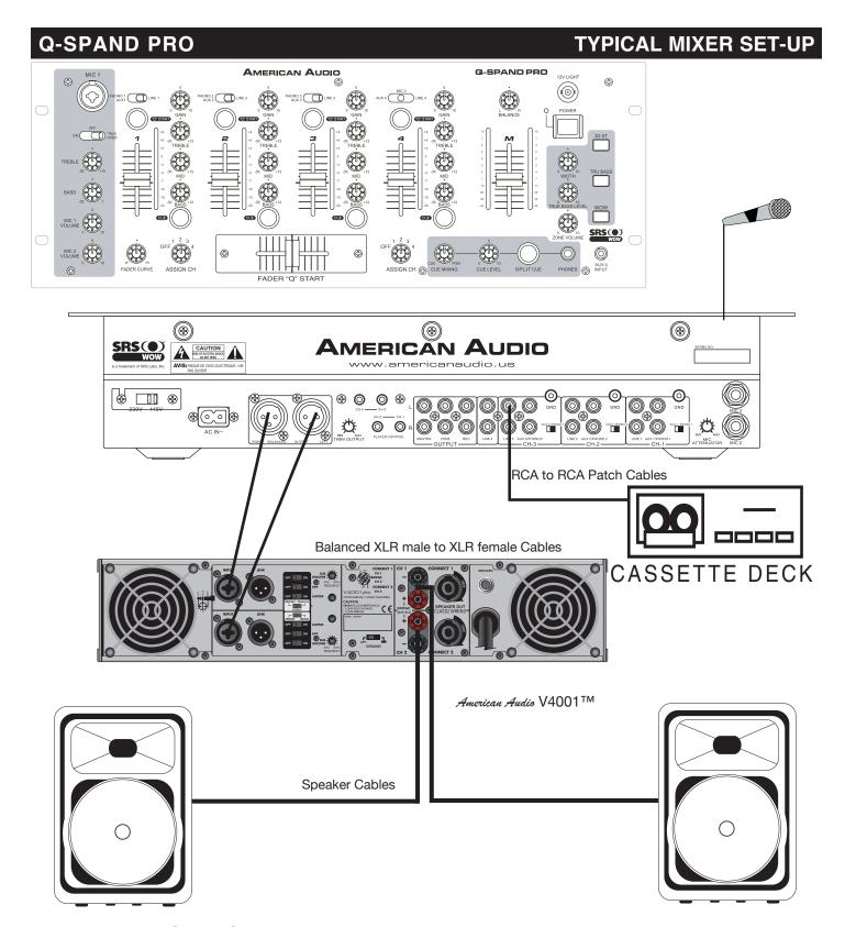
Typical Balanced Output Set-up
