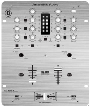
to set the output volume. These controls are used to aid in distortion control. Use these control to preset your signal level before the crossfader. With your channel faders in the maximum position, use the channel trim level to set an average output level of about +4dB on you master level meter.
