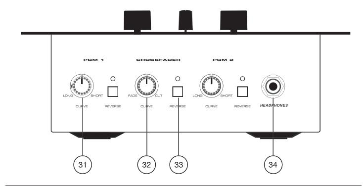
**31. CHANNEL FADER CURVE ADJUSTMENT -** This rotary knob is used to change the way the channel fader will operate. Each of the two channels has a "Curve" adjustment. The curve on the faders adjust from long or short or any variation of the two. The shorter the curve adjustment the sooner full volume will be reached.
