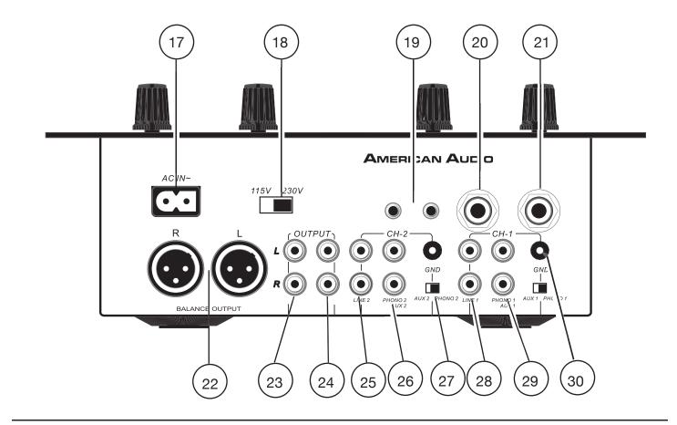
**17. AC CONNECTION -** This connector is used to supply main power to the unit via the included detachable power cord. Use only the supplied, polarized AC power cord. This cord is designed to fit in one direction only. Do not attempt to force a cord in if it does not fit, be sure the cord is being inserted properly
