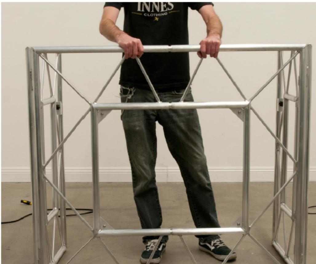
4. Secure both table sections together by installing (2) black metal table support bars. Insert square ends of each support bar into the slots on each side of the table. Insert the front bar first then insert the back bar. Make sure each support bar is completely inserted into the slots and make sure both table sections are level and sitting on a flat surface.
