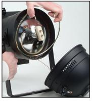
4. Squeeze the lamp retainer ring together and remove it and "free" the lamp.
