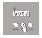
Repeat steps 2-4 in Self Test mode to select desired DMX address.
