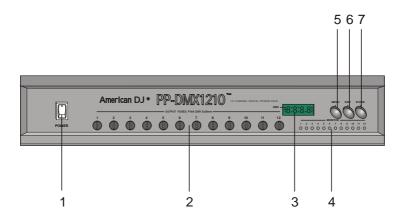
1. Power Switch: Turn on or off the main power of the unit.
