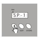
Tap the Menu button, the Segment Display shows "SP" followed by one number 1-9, which indicates Self Test mode is active. A value of 1 gives the slowest speed and the value of 9 gives the fastest speed.
