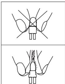
**Halogen Lamp Warning:** This fixture is fitted with halogen lamps which are highly susceptible to damage if improperly handled. Never touch the lamps with your bare fingers as the oil from your hands will shorten lamp life. Also, never move the fixture until the lamps have had ample time to cool. Remember, lamps are not covered under warranty conditions.
