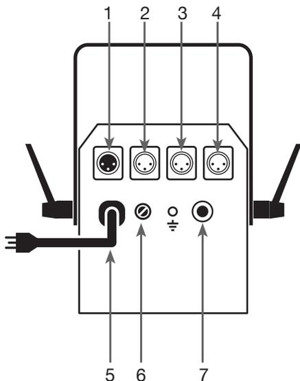
1. **Remote Control Input** - *Do not attempt to connect an audio signal to this jack, this will damage the unit!* This jack is for use with the Luna4/C controller only. *Connecting an audio signal this jack, this will damage the PC board and void your manufactures warranty!*
