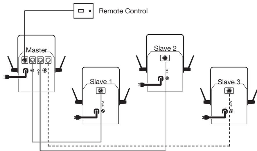
**Linking System:** Your Luna 4™ system comes with built-in programs for a four unit system. Follow the step above for proper linking and set-up procedures. If the system is not set up completely, black spots will appear in the programs.
