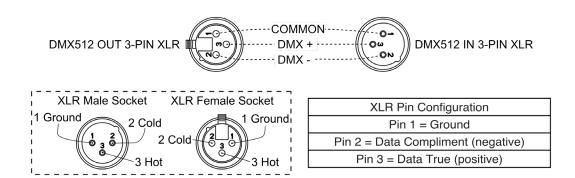
**Special Note:** Line Termination. When longer runs of cable are used, you may need to use a terminator on the last unit to avoid erratic behavior. A terminator is a 110-120 ohm 1/4 watt resistor which is connected between pins 2 and 3 of a male XLR connector (DATA + and DATA -). This unit is inserted in the female XLR connector of the last unit in your daisy chain to terminate the line. Using a cable terminator (ADJ part number Z-DMX/T) will decrease the chances of erratic behavior.
