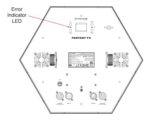
The error indicator LED show different sequences to indicate different fixture errors, as described in the table below:
