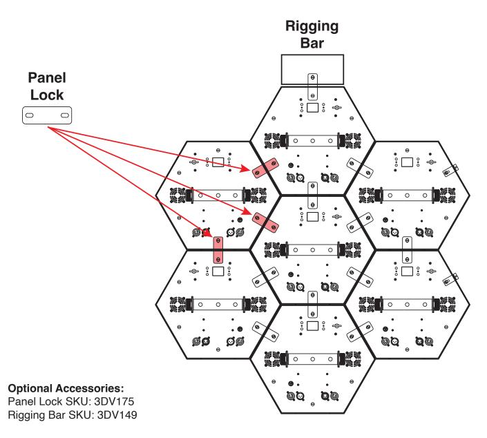
The unit is fully operational in three different mounting positions: hanging upside-down from the ceiling or trussing, or sideways on trussing. Be sure this fixture is kept at least 1m (3.3 ft) away from any flammable materials (decorations, etc). Always use and install a safety cable (not included) as a safety measure to prevent accidental damage and/or injury in the event the clamp fails.
