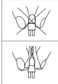
This fixture is fitted with halogen lamps which are highly susceptible to damage if improperly handled. Never touch lamp with your bare fingers as the oil from your hands will shorten lamp life. Also, never move the fixture until the lamps have had ample time to cool. Remember, lamps are not covered under warranty conditions.
