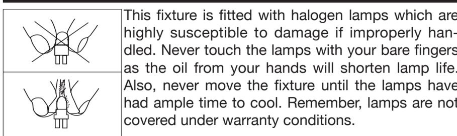
This fixture is fitted with halogen lamps which are highly susceptible to damage if improperly handled. Never touch the lamps with your bare fingers as the oil from your hands will shorten lamp life. Also, never move the fixture until the lamps have had ample time to cool. Remember, lamps are not covered under warranty conditions.
