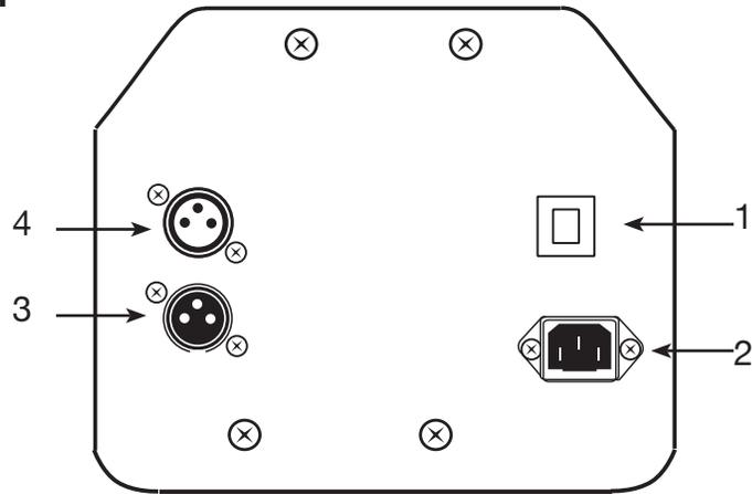
**1. Breaker** - A 5A built-in safety breaker to reduce the risk of electrical shock or fire and protect the circuitry. In the case of an internal short or power surge.
