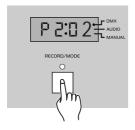
Tap the Mode button several times until both Manual and Audio LEDs go out, that is, Auto mode is active.
