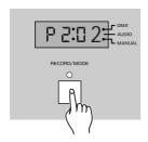
Tap the Mode button several times until the a dot LED near Manual lights.
