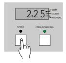
Tap the Speed or Fade+Speed button to select chase mode or fade mode, the LED above it lights indicating your selection.
