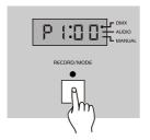
Press and hold down the Record/Mode button for five seconds, the LED above it lights indicating Record mode is active, the Segment Display shows the program and its scene of last time.
