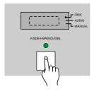
Tap the Fade+Speed button to send file dump.
