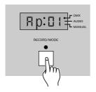
Create a scene on your DMX controller, tap the Record button, all LEDs flash briefly indicating you've record a scene(step) into this program.
