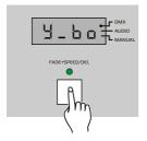
3. Tap the Fade+Speed button to change between "N-BO" and "Y-BO".
