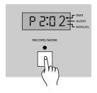
3. Create a scene on your DMX controller, tap the Record button, all LEDs flash briefly indicating you've added a scene(step) into this program.
