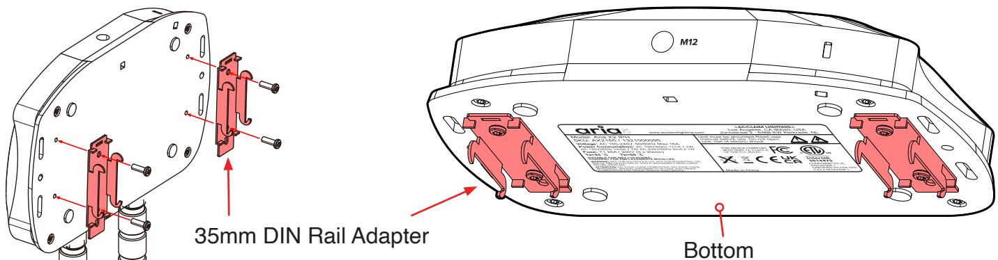
2. Mount the Aria X2 Transceiver by aligning the 35mm DIN Rail Adapters with the slots on the 35mm DIN rail. Slide the Aria X2 Transceiver onto the rail until it clicks or locks into place securely.
