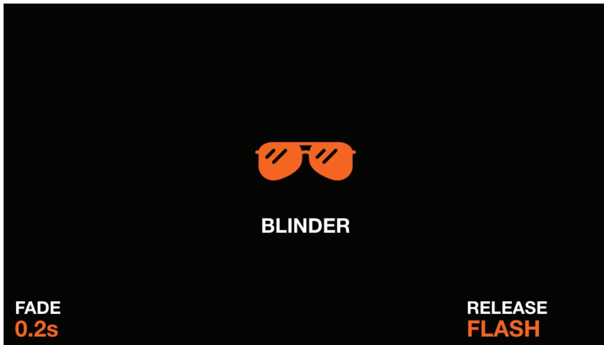
The Blinder flash effect sets all dimmers to 100% and all color mixing channels to white. The effect is released according to the set release mode.
