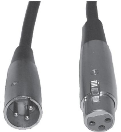
**Notice:** Be sure to follow figures two and three when making your own cables. Do not use the ground lug on the XLR connector. Do not connect the cable’s shield conductor to the ground lug or allow the shield conductor to come in contact with the XLR’s outer casing. Grounding the shield could cause a short circuit and erratic behavior.
