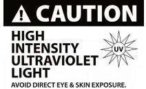
RISK GROUP 3 - RISK OF EXPOSURE TO ULTRAVIOLET UV RADIATION! FIXTURE EMITS HIGH INTENSITY WAVELENGTH OF ULTRAVIOLET UV LIGHT FROM THE UV COLOR FILTER. WEAR PROPER EYE AND SKIN PROTECTION. AVOID PROLONGED PERIODS OF EXPOSURE TO UV COLOR FILTER. AVOID WEARING WHITE COLOR CLOTHING AND/OR USING UV PAINTS ON SKIN. AVOID DIRECT EYE AND/OR SKIN
