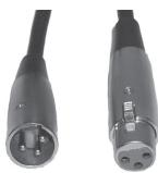
**Notice:** Be sure to follow the figures below when making your own cables. Do not use the ground lug on the XLR connector. Do not connect the shield of the cable conductor to the ground lug, or allow the shield conductor to come in contact with the outer casing of the XLR. Grounding the shield could cause a short circuit and erratic behavior.
