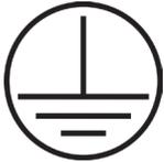
**CLASSE DE PROTECTION 1 - LE LUMINAIRE DOIT ÊTRE CORRECTEMENT MISE À LA TERRE**
