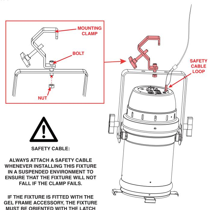
FACING UPWARDS. THIS IS TO PRE-VENT THE GEL FRAME FROM FALLING IN THE EVENT THAT THE LATCH FAILS.
