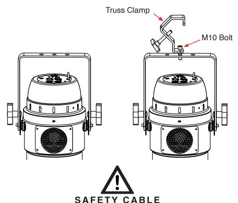
ALWAYS ATTACH A SAFETY WHENEVER INSTALLING THIS FIXTURE IN A SUSPENDED ENVIRONMENT TO ENSURE THE FIXTURE WILL NOT FALL IF THE CLAMP FAILS. CLAMP INSTALLATION
