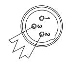
A DMX512 terminator reduces signal errors, avoiding most signal reflection interference. Connect PIN 2 (DMX-) and PIN 3 (DMX+) of the last fixture in series with a 120 Ohm, 1/4 W Resistor to terminate the DMX512.
