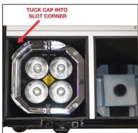
4. Place an ADJ Mirage Q IP device in any of the device slots in the flight case. Up to 6 devices can be accommodated. The charge indicator located beside the power ports will illuminate to indicate that your device is charging. It is strongly recommended to leave the case lid open during charging.
