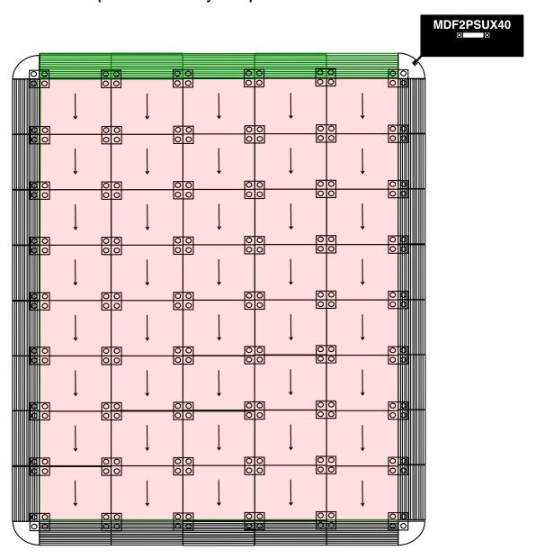
**NOTE:** Directional orientation arrows are depicted on the top surface of the panels for the sake of clarity. Actual panels will have directional orientation arrows located on the sides of the panels.
