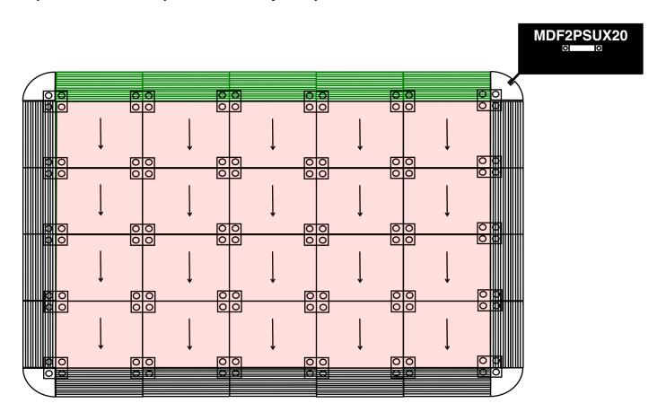
**NOTE:** Directional orientation arrows are depicted on the top surface of the panels for the sake of clarity. Actual panels will have directional orientation arrows located on the sides of the panels.
