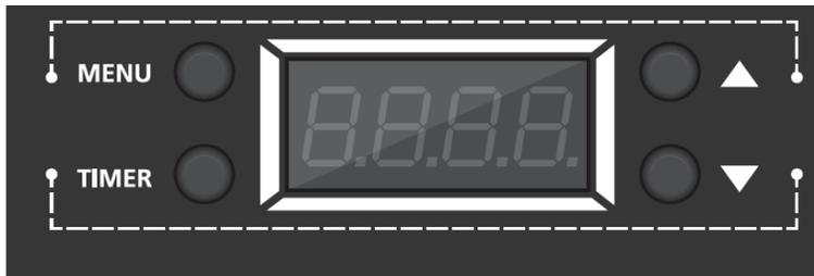
**MENU BUTTON** - Press this button to cycle between DMX addressing, fan adjustment, duration adjustment, and interval adjustment. Use the UP and DOWN buttons to make your desired adjustments.
