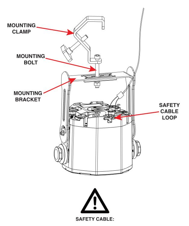
ALWAYS ATTACH A SAFETY CABLE WHENEVER INSTALLING THIS FIXTURE IN A SUSPENDED ENVIRONMENT TO ENSURE THAT THE FIXTURE WILL NOT FALL IF THE CLAMP FAILS.
