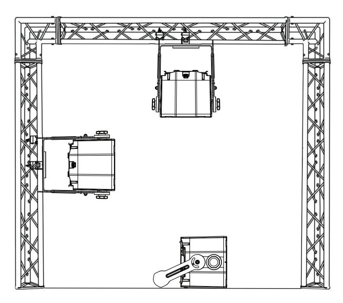
The unit is fully operational in three different mounting positions: hanging upside-down from the ceiling or trussing, sideways on trussing, or set on a flat level surface. Be sure this fixture is kept at least 12m (40ft) away from any flammable materials (decorations, etc). Always use and install a safety cable (not included) as a safety measure to prevent accidental damage and/or injury in the event the clamp fails. Never use the carrying handles for secondary attachment.
