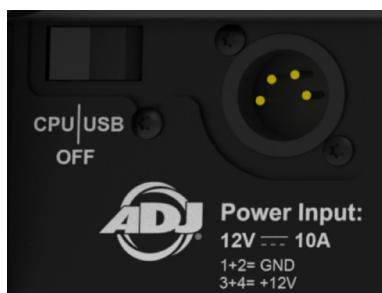
2. Insert the 4-pin XLR connector from the external power supply unit into the power input on the back of the console.
