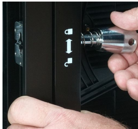
1. Align the locking-tab with tab-keyed connector socket
