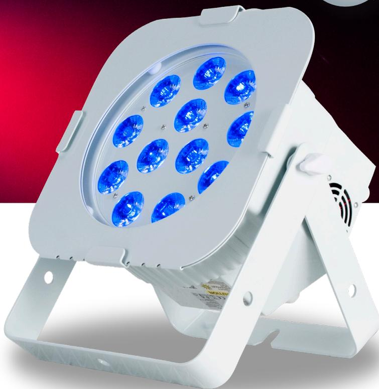
The ADJ 12PX HEX Pearl is a versatile LED Par fixture with 12 x 12-Watt, 6-IN-1 HEX LEDs made from all metal construction. With a 25-degree beam angle, users may produce wide washes with smooth color mixing from 63 built-in color macros utilizing red, green, blue, amber, white and UV LEDs. Not only is this LED Par great for lighting stages, but with its patent pending, intelligently designed, power and DMX connectors, it's great for uplighting a venue or used as a stage wash.
